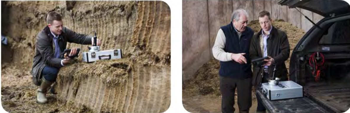
Figure 2: Portable NIR being used for Forage analysis on farm
